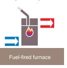
**Furnaces** – a furnace burns fuel (natural gas, propane, oil) to generate heat in a combustion chamber. Heat from the combustion chamber is transferred through a heat exchanger to air inside the home. It is critical that the furnace be properly vented to
