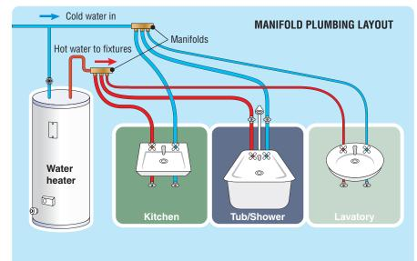
A plumbing manifold system provides cutoff valves at the main terminus with flexible plumbing hoses that connect to the fixtures. Insulating the manifold and connecting lines is critical to reduce standby losses.
