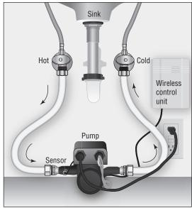
An on-demand hot water distribution system can be installed easily in new homes. As a retrofit solution, an on-demand pump can be installed at the furthest fixture from the water heater. A do-it-yourselfer can install such a unit under a lavatory sink. It involves shutting off the water main, adding hose "T" extensions to the cut-off valves and connecting bypass hoses to the pump (note: a GFCI electrical outlet is required to power the pump).
